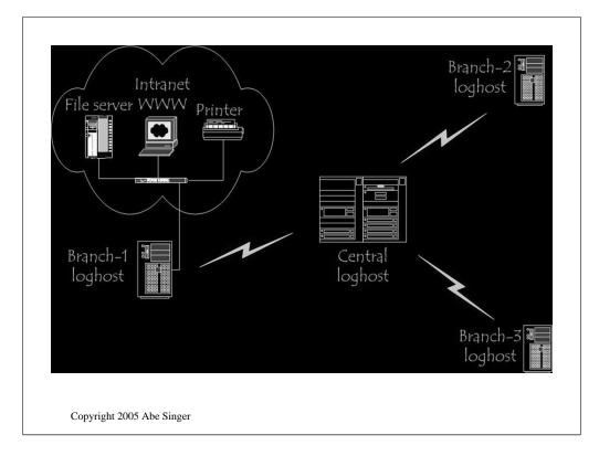
diagram of a relay architecture
